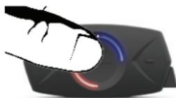
Press and hold the multi-function button until the status indicator turns blinking red/blue on each **SHARKTOOTH**.
