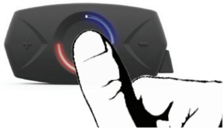
Press and hold the multi-function button until the status indicator turns blinking red/blue.
