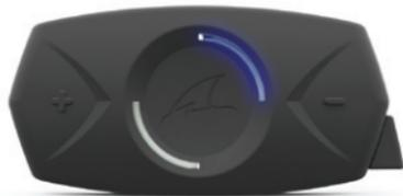
When the status indicator turns blinking blue, the pairing is successful!
